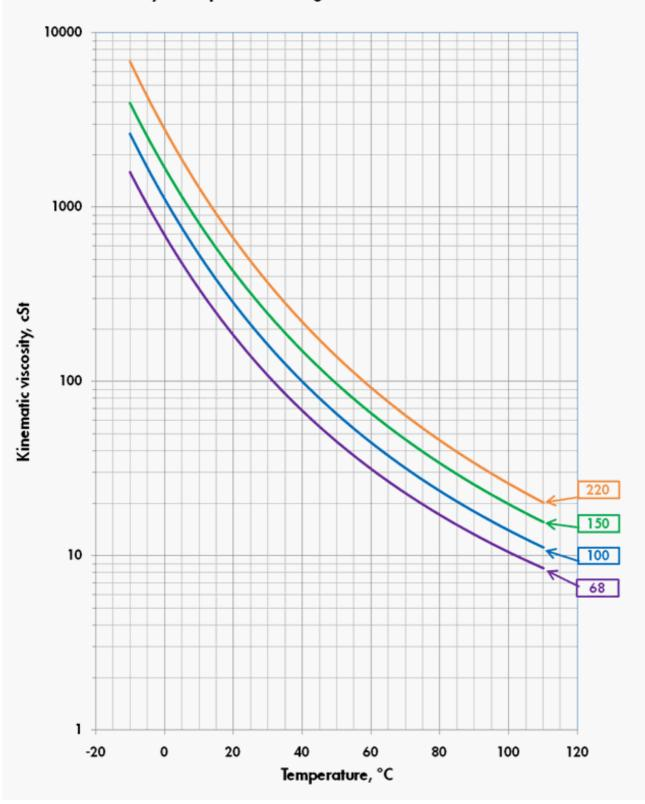
Viscosity - Temperature Diagram for Shell Morlina S4 B
