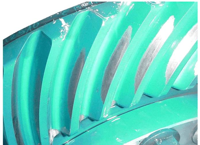
Load-bearing pattern made visible on a bevel gear.
