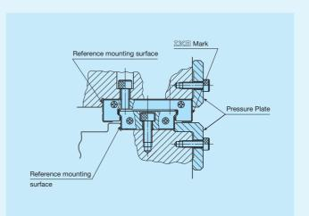
Fig. 2 Mounting example when lateral load is the primary load
