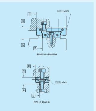
Fig. 1 Reference mounting surface and mounting examples
